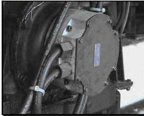
Fig.8 : The wheel sensor installation
