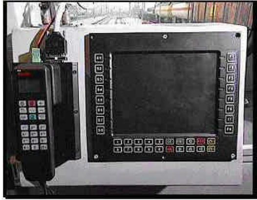
Fig.5 : The DMI and handset installation
